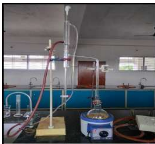
Fig 1. Extraction of Essential Oil by Clevenger Method
