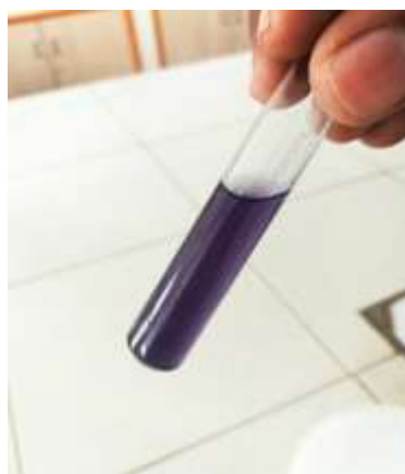
Figure 2: Confirmatory test for anthocyanins using HCl — stable purple colouration at 100°C.
