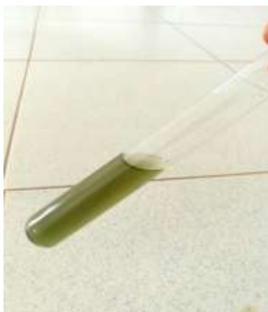
Figure 3: Confirmatory test for anthocyanins using NaOH — characteristic green colour.
