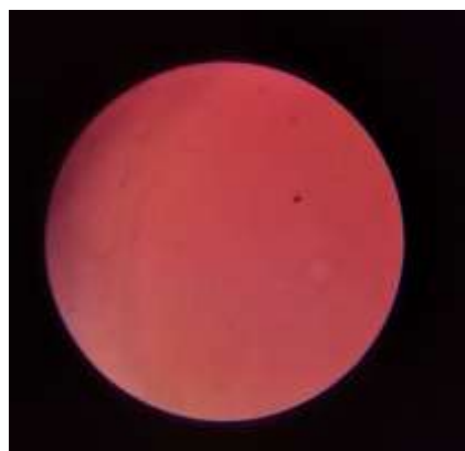
Figure 3. Dye test showing the O/W emulsion
