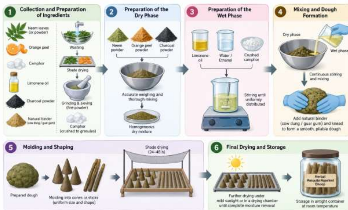
Figure 2. Illustration of the stepwise formulation process of herbal mosquito repellent dhoop
