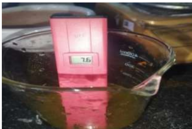
Figure no.4: pH Test of formulation
