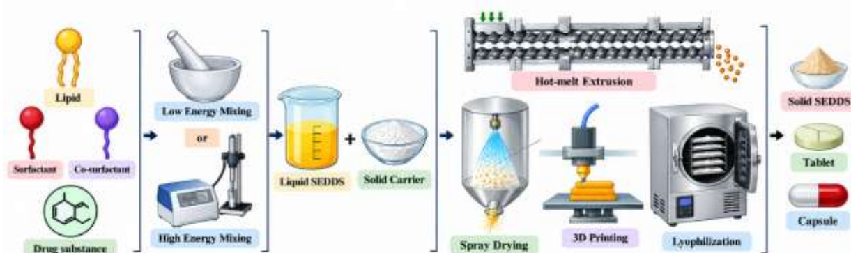
Figure 3. Liquid SEDDS to solid SEDDS using various techniques
