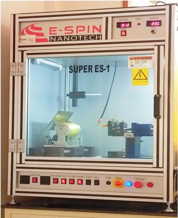
Figure 2: Preparation of Nanofiber by Electrospinning Technique.
