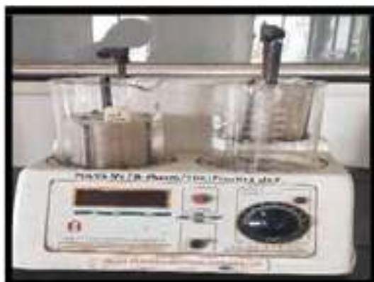
Fig No. 2 Disintegration time apparatus
