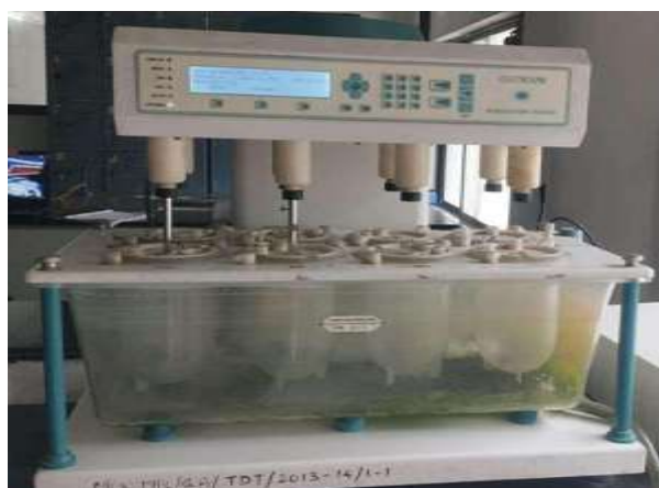
Fig No. 3 Dissolution Test Apparatus
