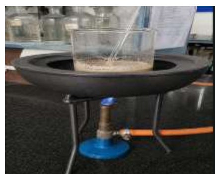
Fig no :5 Heating of powder with ethanol water (1:2)
