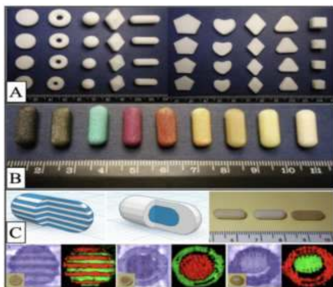
Figure 3. Images of various types of tablets prepared by FDM technology: (A) Images of 3D-printed tablets with different shapes and sizes [84]; (B) images of 3D-printed tablets in capsule form with different colors [84]; (C) sectioned multilayer device and sectioned DuoCaplet (caplet in caplet) model images, 3D-printed preparations, and white light and 2-dimensional Raman mapping images [85].
